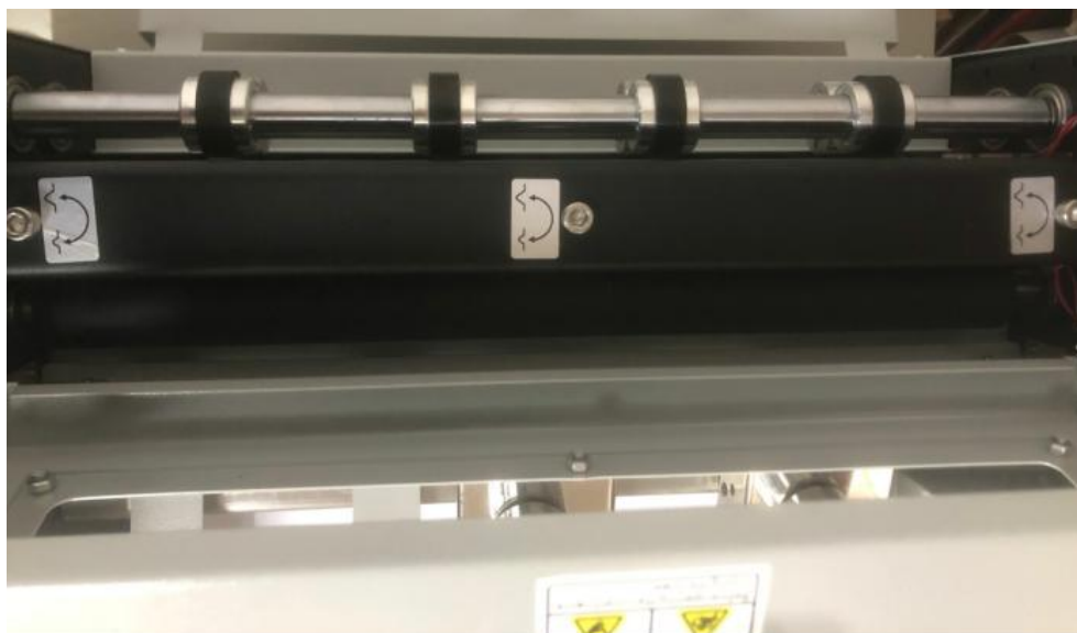
3 Creasing depth adjusting screws
